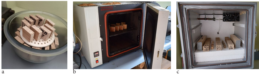
Figure 3. Exposure of experimental samples in different temperature and humidity conditions
