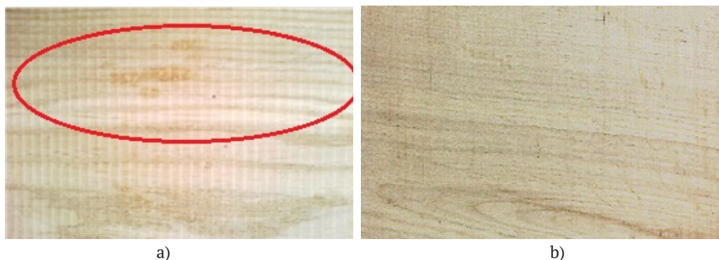
Figure 3. The surface of lamella made of oak wood, dried in various modes: a) low-temperature with the presence of white spots; b) cyclic – with a uniform colour
