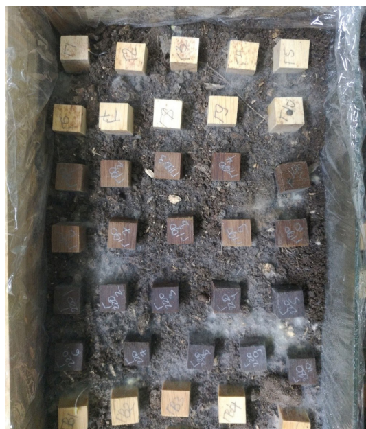
Figure 7. Changing the appearance of hornbeam wood samples after a week of exposure in a soil box
