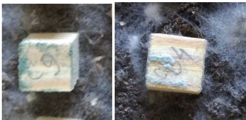
Figure 6. View of pine wood samples on Day 6 of the exposure in a box with soil: a – untreated; b – surface is treated with wax oil
