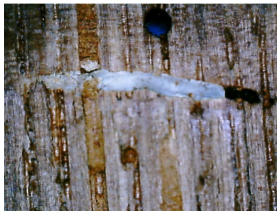
Figure 3. Timber pest passages within the wood
