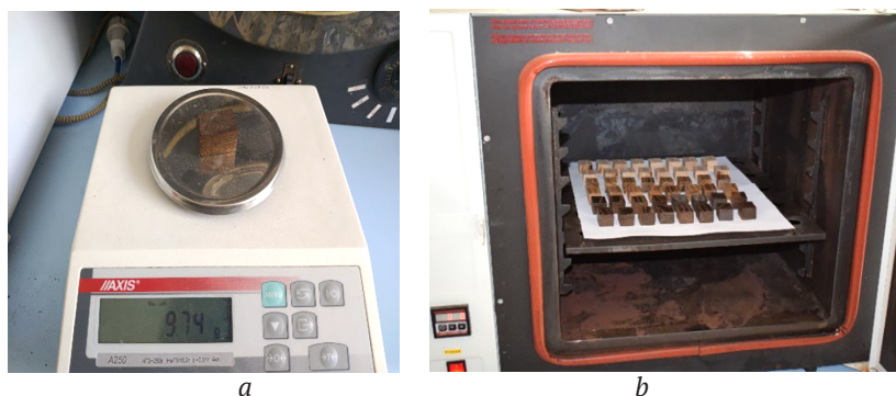
Figure 5. Example of weighing (a) and drying of test samples (b)
