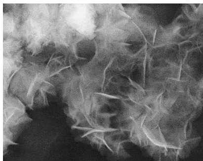
Figure 3. View of magnesium nanoparticles through a Zeiss SUPRA 40VP electron microscope (SEM)
