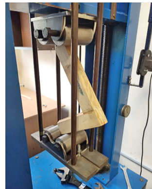
Figure 6. Structure for destructive testing of corner joints
