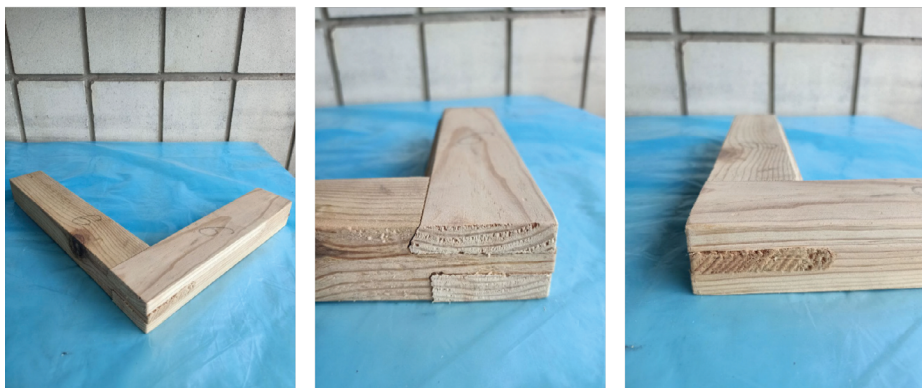
Figure 3. Connecting parts through a tongue
