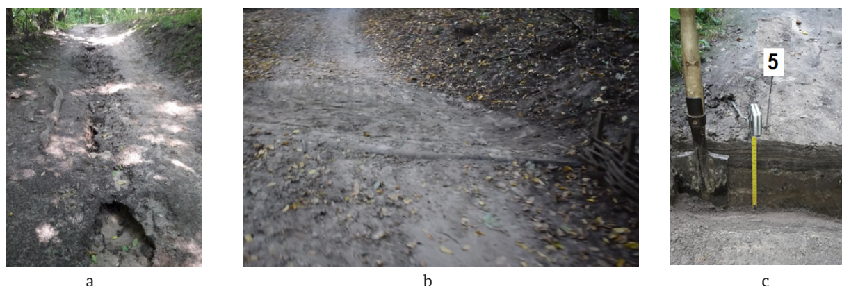
Figure 4. Characteristic erosion processes on park paths were identified: a – linear erosion; b – scum on the drain sprayer; c – the thickness of washed soil for 2021-2022
