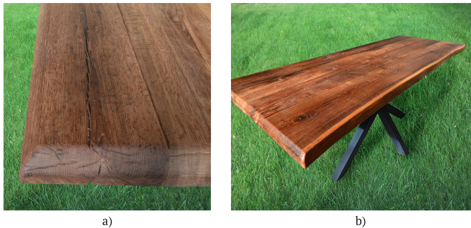
Figure 7. Table made of thermally modified oak wood: a – part of the tabletop that shows the passages of insects; b – general view of the table
