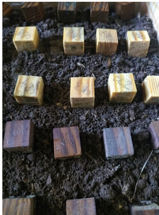
Figure 9. Appearance of black spots on oil-waxed pine wood samples on Day 24
