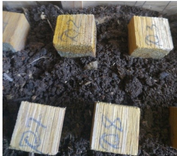
Figure 8. View of untreated oak wood after two weeks of research
