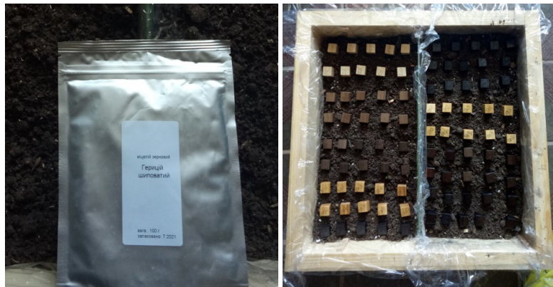
Figure 4. Determination of wood resistance to biological pests: a – cultures of fungi Hericium erinaccus ; b – experimental samples of wood in laboratory conditions
