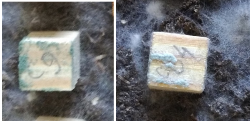
Figure 6. View of pine wood samples on Day 6 of the exposure in a box with soil: a – untreated; b – surface is treated with wax oil
