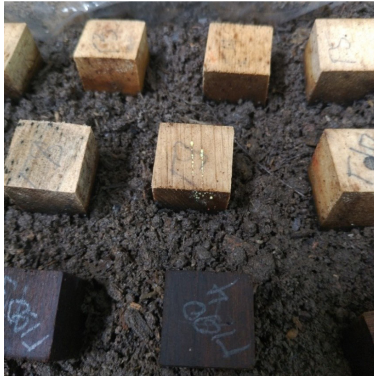
Figure 10. Appearance of untreated hornbeam samples on Day 38 of exposure under aggressive conditions
