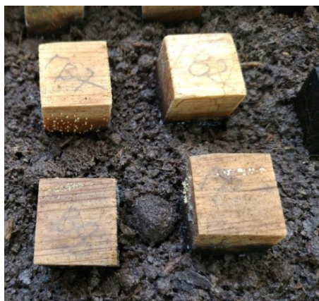
Figure 11. Appearance of hornbeam wood samples treated with wax oil
