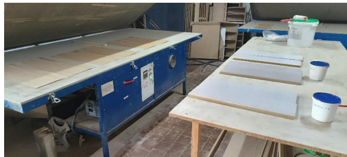
Figure 2. Experimental samples with an MDF/chipboard base are faced with oak veneer using glues of various degrees of water resistance
