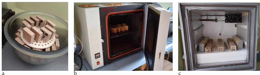
Figure 3. Exposure of experimental samples in different temperature and humidity conditions Note: a – humid environment, b – high temperature ( 80 \pm 2^\circ\text{C} ), c – low temperature ( -15 \pm 3^\circ\text{C} )
