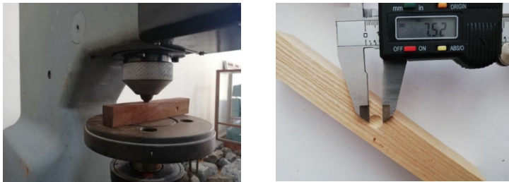
Figure 2. Visualisation of static hardness tests of ash wood samples Source: compiled by the authors
