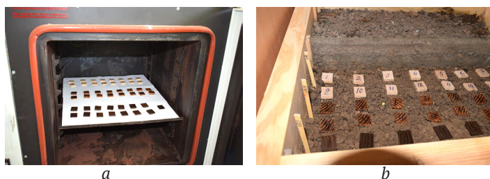
Figure 4. Placement of samples for decay resistance testing
