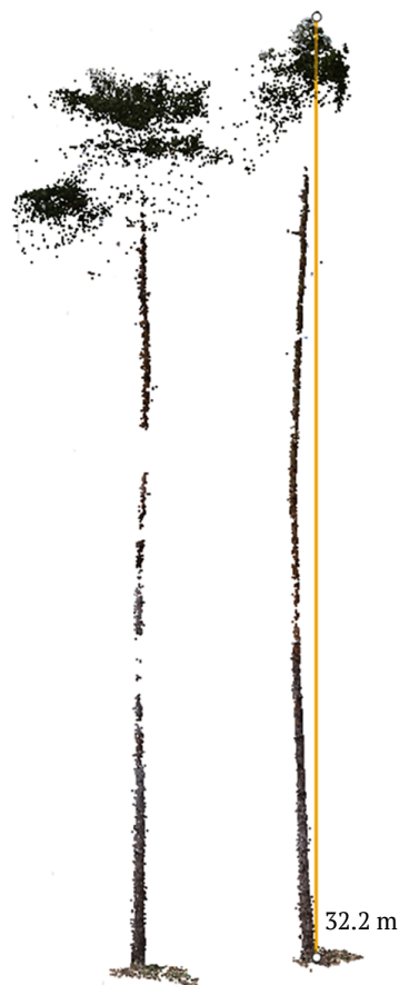
Figure 1. Height measurement from a point cloud (PC method)
