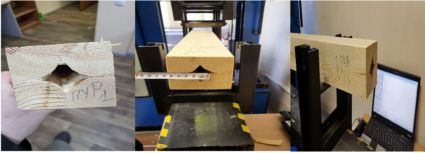
Figure 1. Experimental specimens with a central cavity formed by a debarked surface Source: compiled by the author on the basis of experimental research
