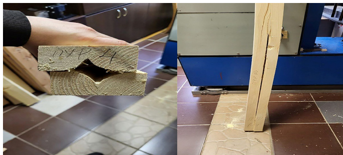
Figure 4. Adhesive fracture of the PUR specimen: delamination of the foam
